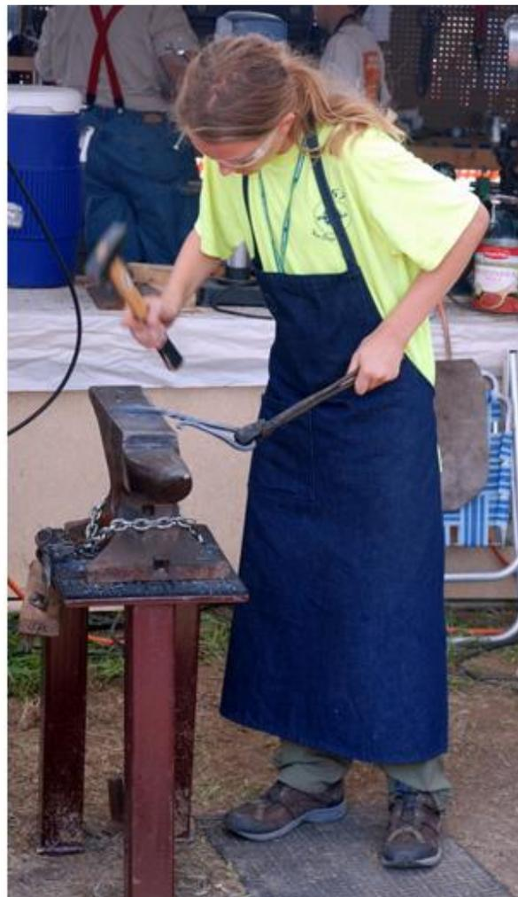
Heated metal held against an anvil is shaped with blows from a blacksmith's hammer. As the metal cools, it is returned to the forge to be heated again.
